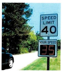
Speed limit feedback signs provide the driver with real-time information related to their speed. These devices do positively affect speed limits, but still rely on driver compliance.
