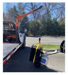
Crane. Mounted a crane on the F-450 pickup, to quickly and efficiently clear large items (such as trees), replace damaged signs, and transport heavy equipment.
